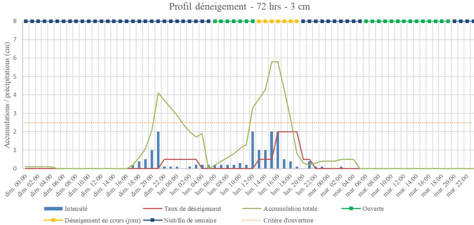
Figure 29 : Profile of snow removal operations over a 72-hour period (between 7 and 9 January 2018, acceptability criterion of 3 cm)
