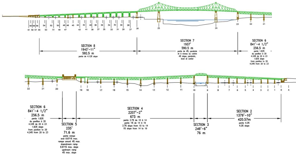
Figure 1 : Schematic representation of the bridge profile (not to scale)
