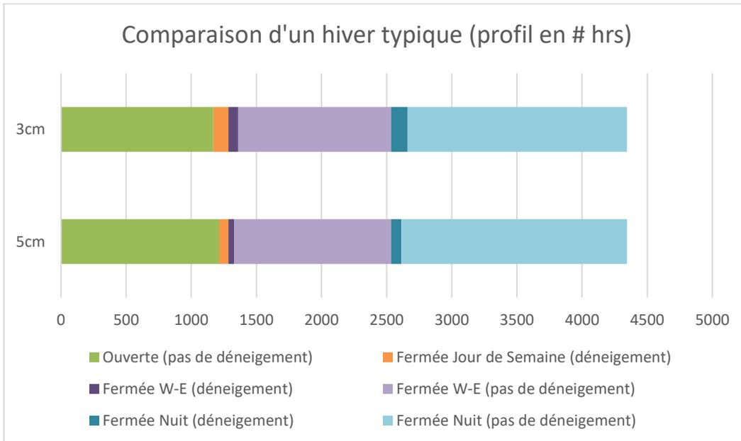
Figure 36 : Comparison of a typical winter (number of hours) by modifying the acceptability criterion from 3 to 5 cm.
