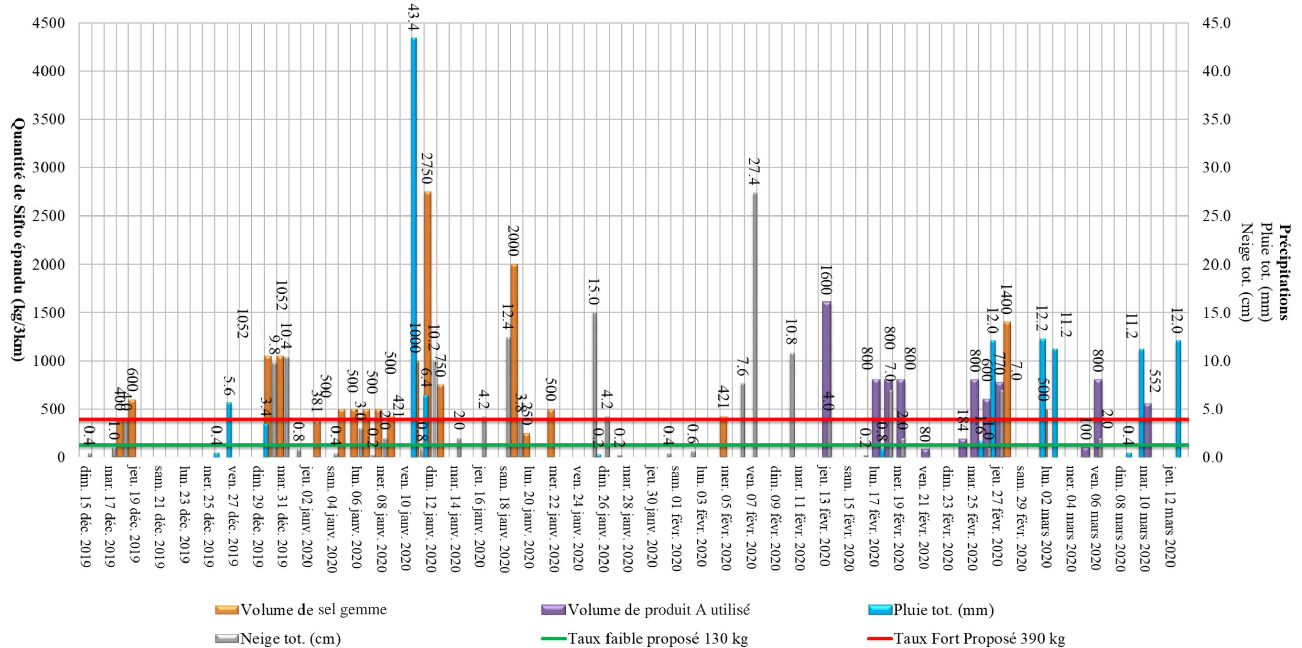
Figure 11 : De-icing application rates and precipitation during the winter of 2019-2020
