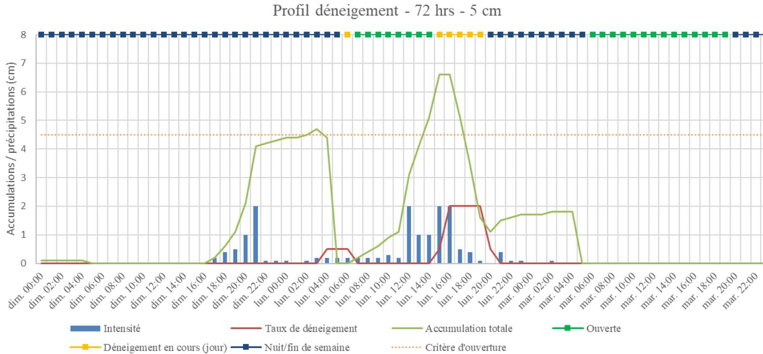
Figure 30 : Profile of snow removal operations over a 72-hour period (between 7 and 9 January 2018, 5 cm acceptability criterion)
