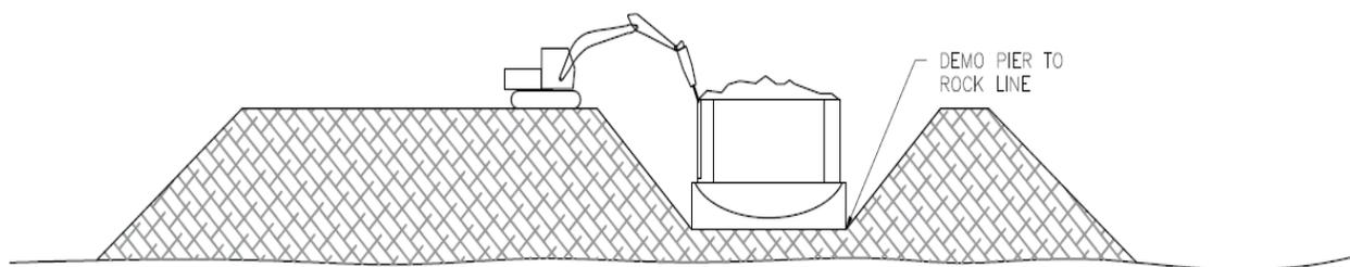
**Figure 16 – Standard demolition of a footing on a temporary jetty**
