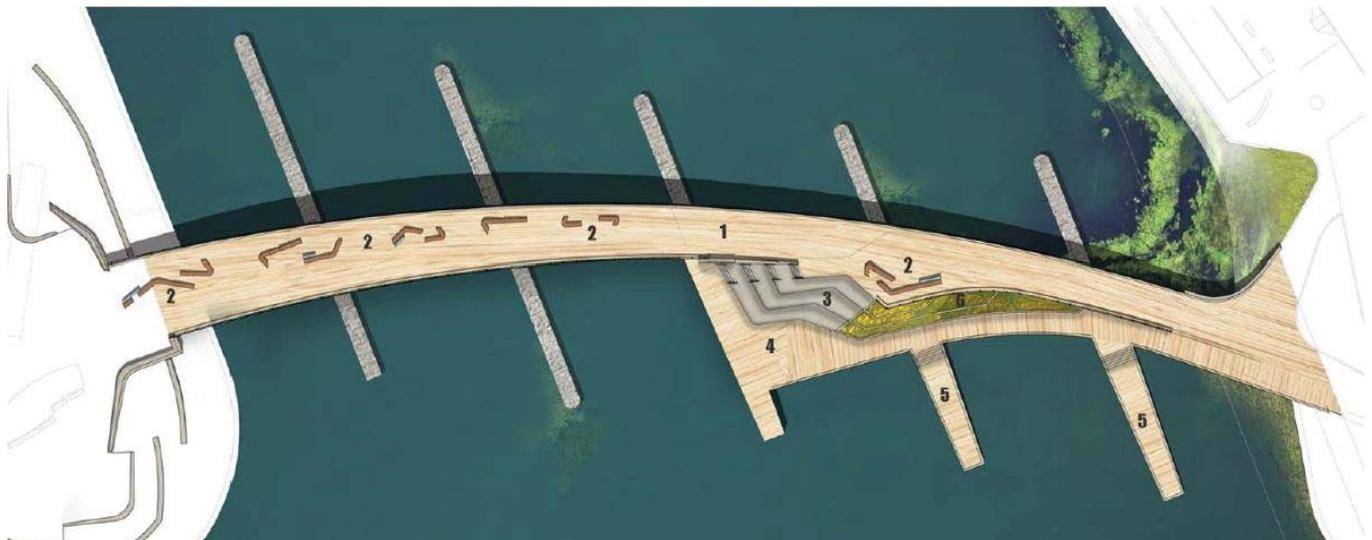
Figure 10 – General layout showing the five concrete pillars from the old bridge. Source: City of Providence, 2014
