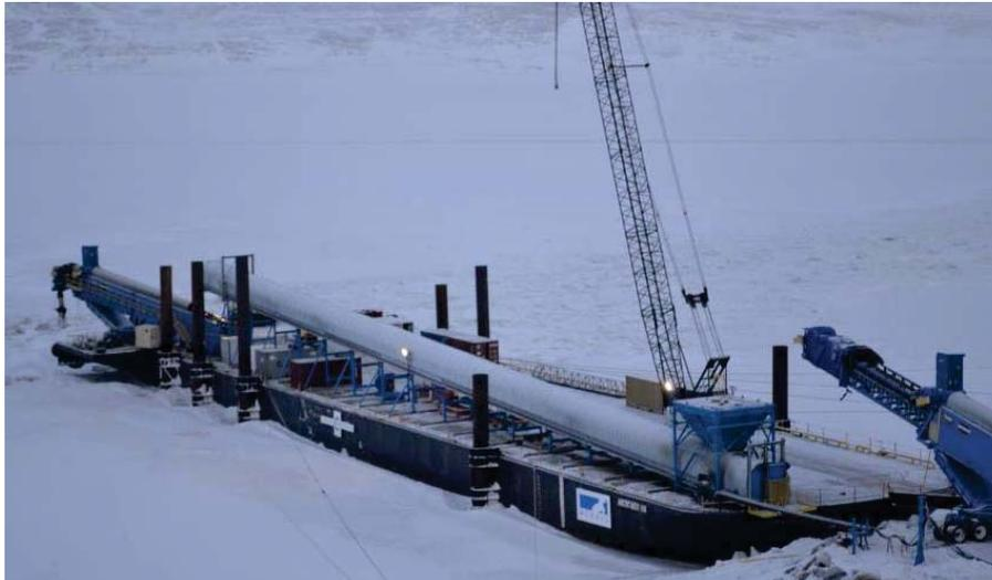
Figure 113 – Barge with “Jack-up” Type Anchored Pillar
