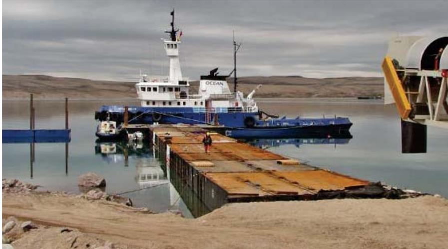
Figure 90 – Sectional Barge
