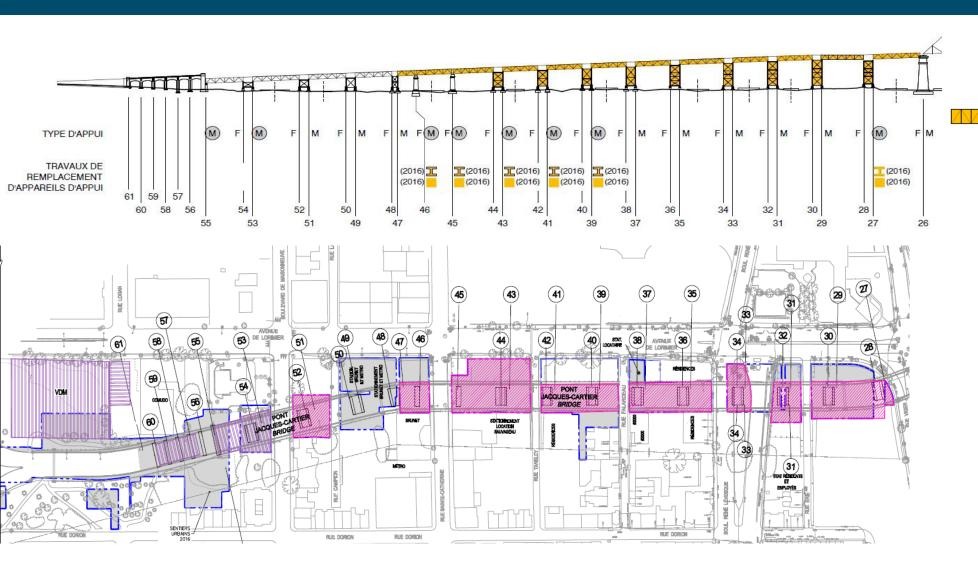
RENFORCEMENT D'ACIER ET REMPLACEMENT DES APPAREILS D'APPUIS
